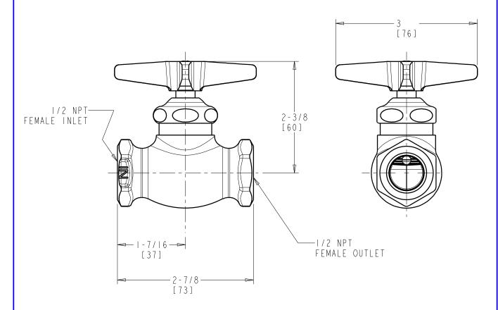
DIMENSIONS ARE IN INCHES AND [MILLIMETERS].
